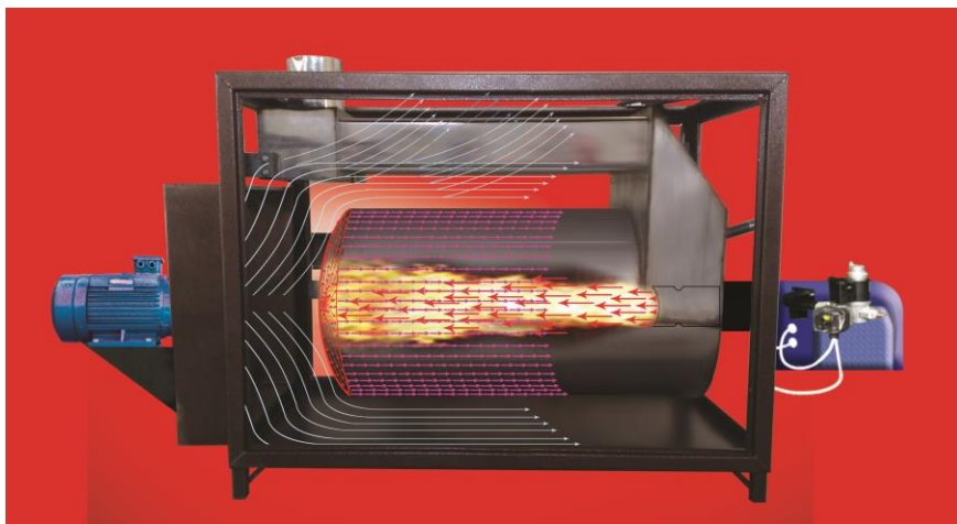
Figure 2- How OASIS 270 heater works
